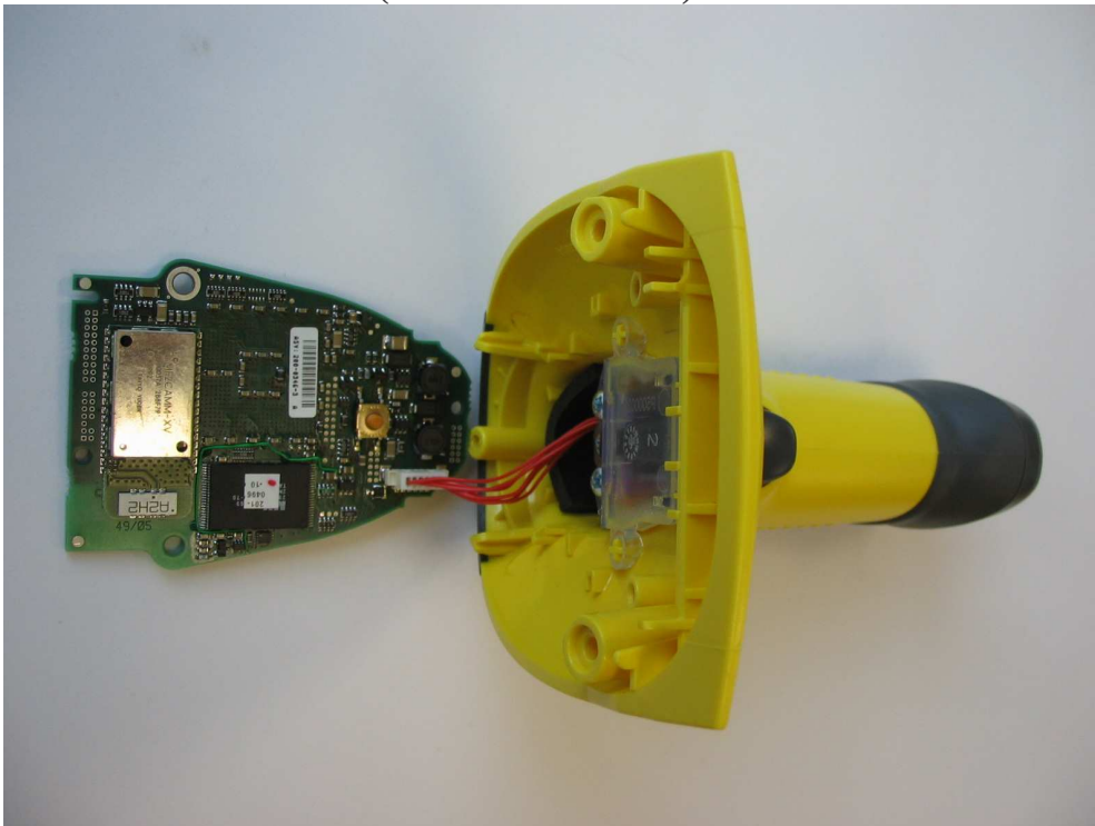
Open 6320 with main board (rear side)
