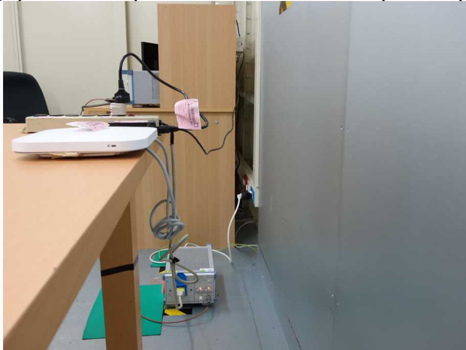
Photograph 20: Test Setup for Mains Conducted Emissions (Back View)
