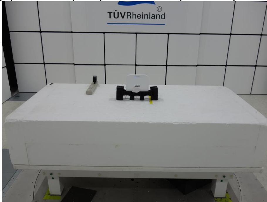
Photograph 8: Test Setup for Spurious Emissions (Front View 2)
