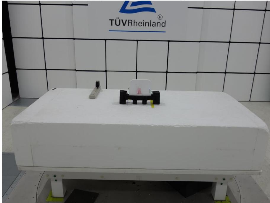
Photograph 1: Test Setup for Spurious Emissions (Front View 1)
