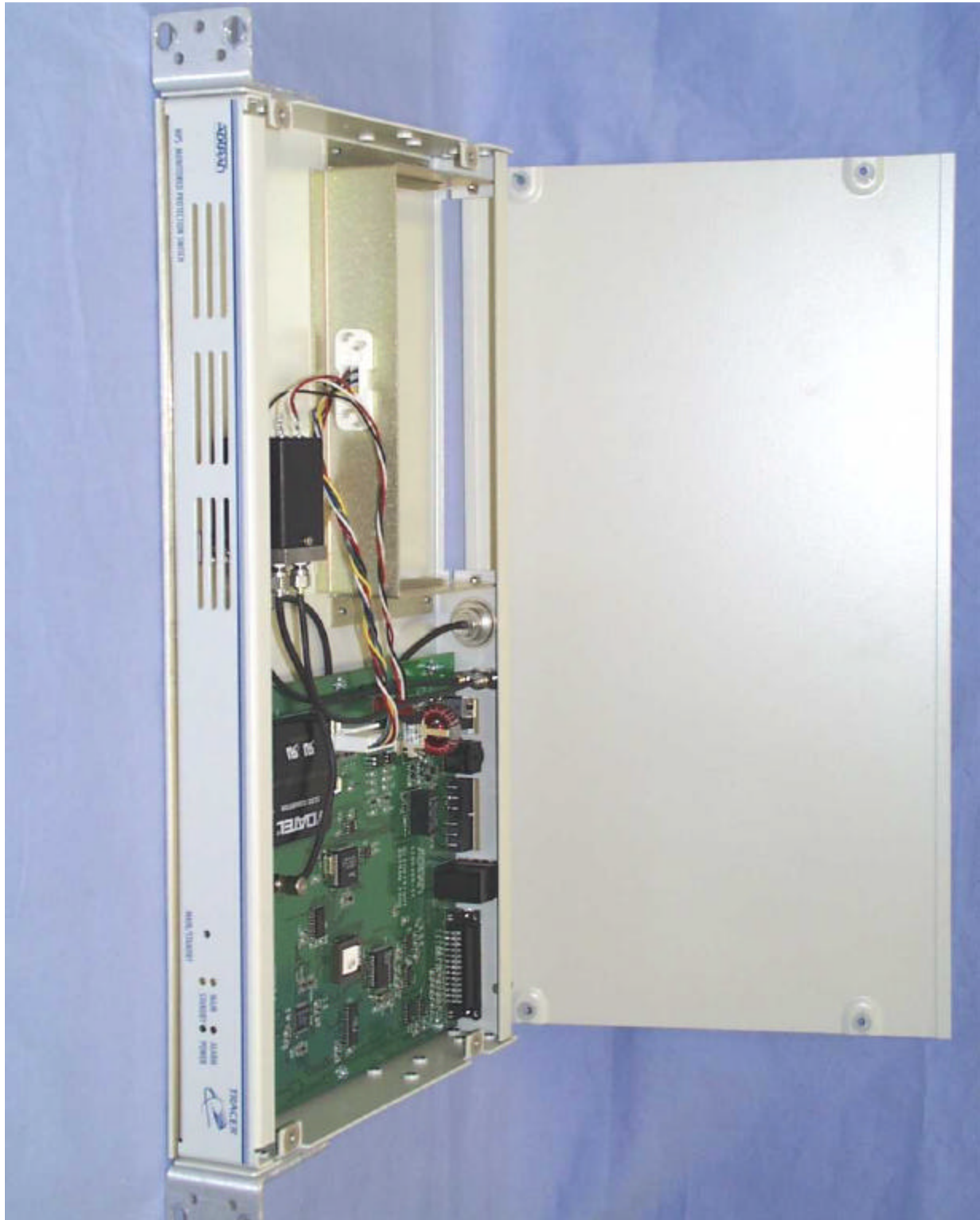
Photograph 2.5 Tracer Monitored Protection Switch Inside Chassis
