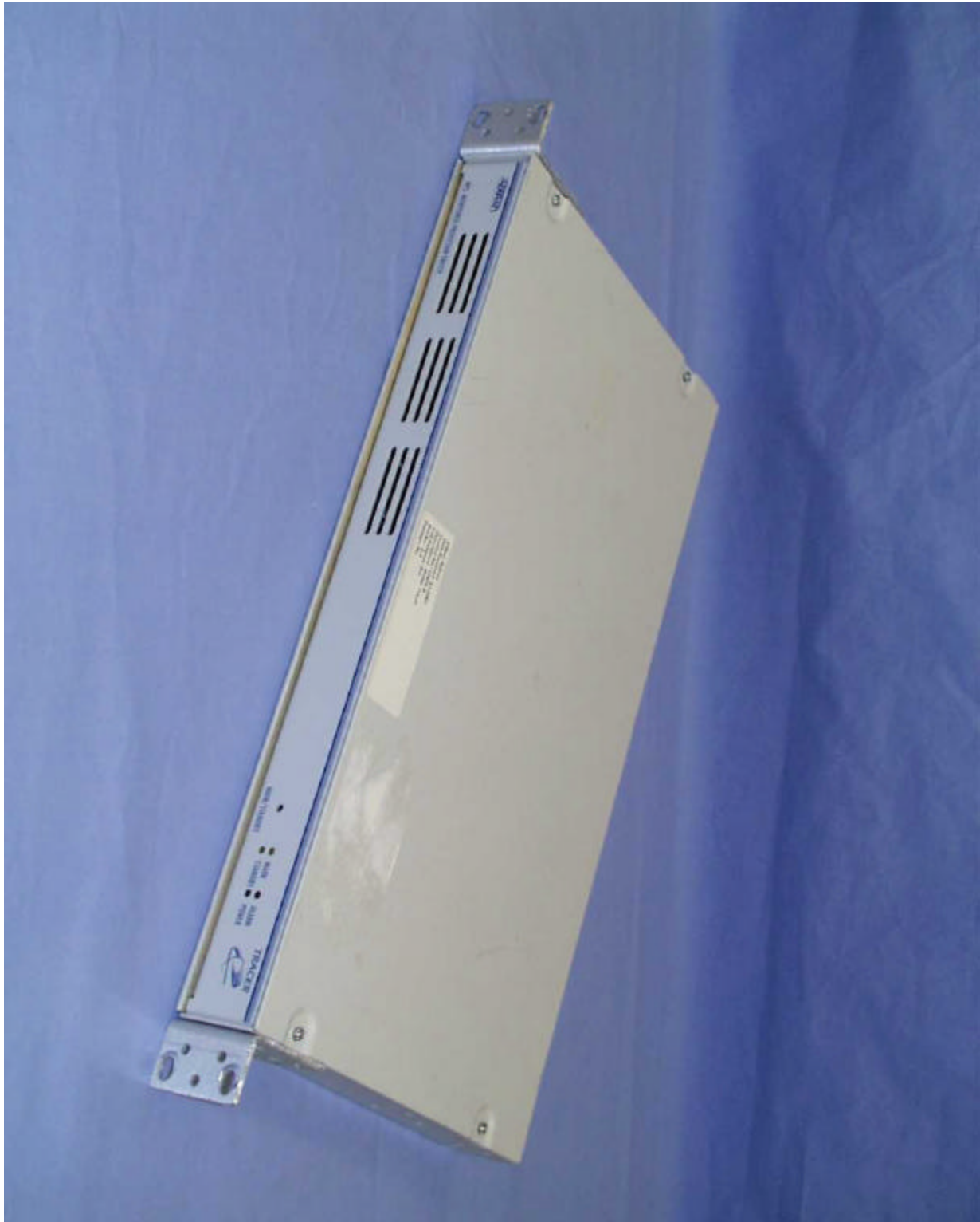
Photograph 2.1 Tracer Monitored Protection Switch Front / Top View
