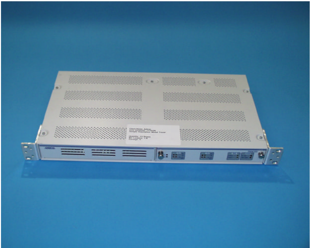
Photograph 4.15: Baseband Processor Assembly Front View
