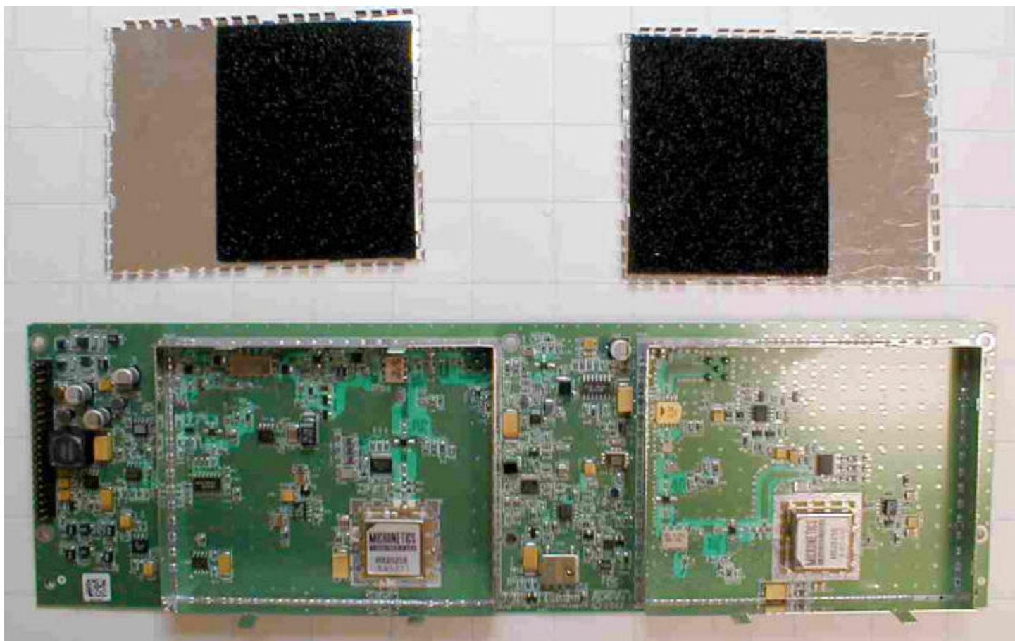
RFC Board Bottom, Shields Removed
