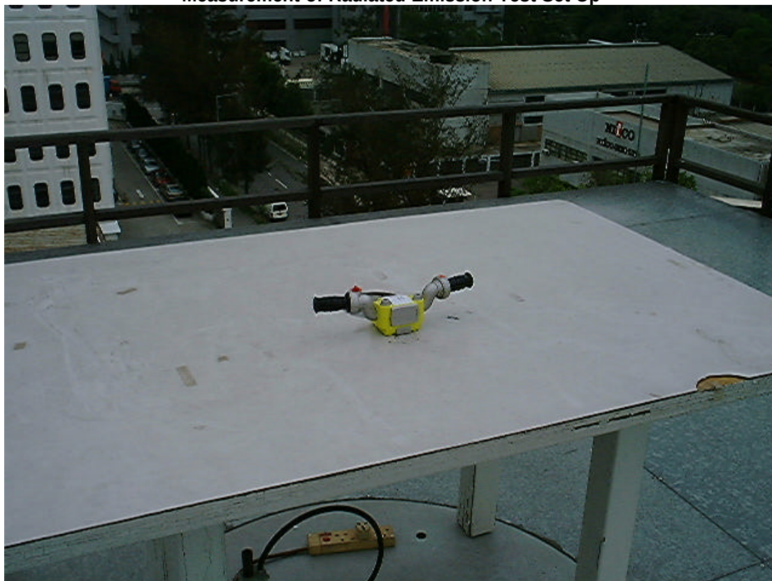
Measurement of Radiated Emission Test Set Up
