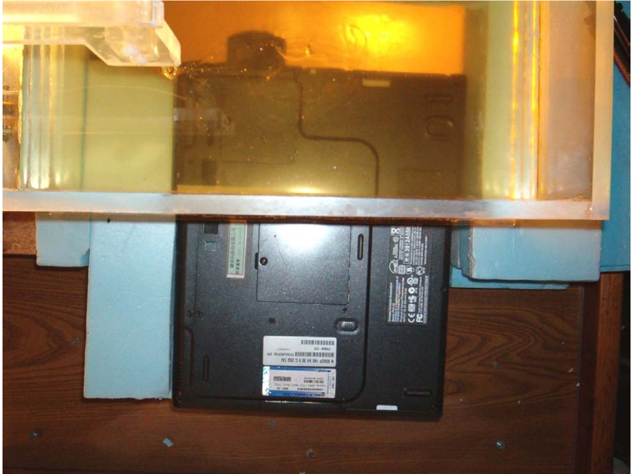
Fig. 5. Photograph of the Accton Technology Corporation WLAN Mobile Adapter inserted into a Compaq laptop computer with its bottom pressed against the bottom of the planar tissue-simulant phantom to simulate "above-lap" placement of the wireless PC. A Styrofoam block is used under the base to prevent bending of the 2 mm thin base of the phantom.
