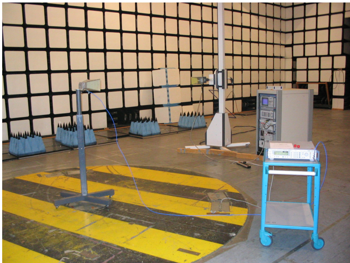
Figure 5-8: Test set-up for the Dipole substitution
