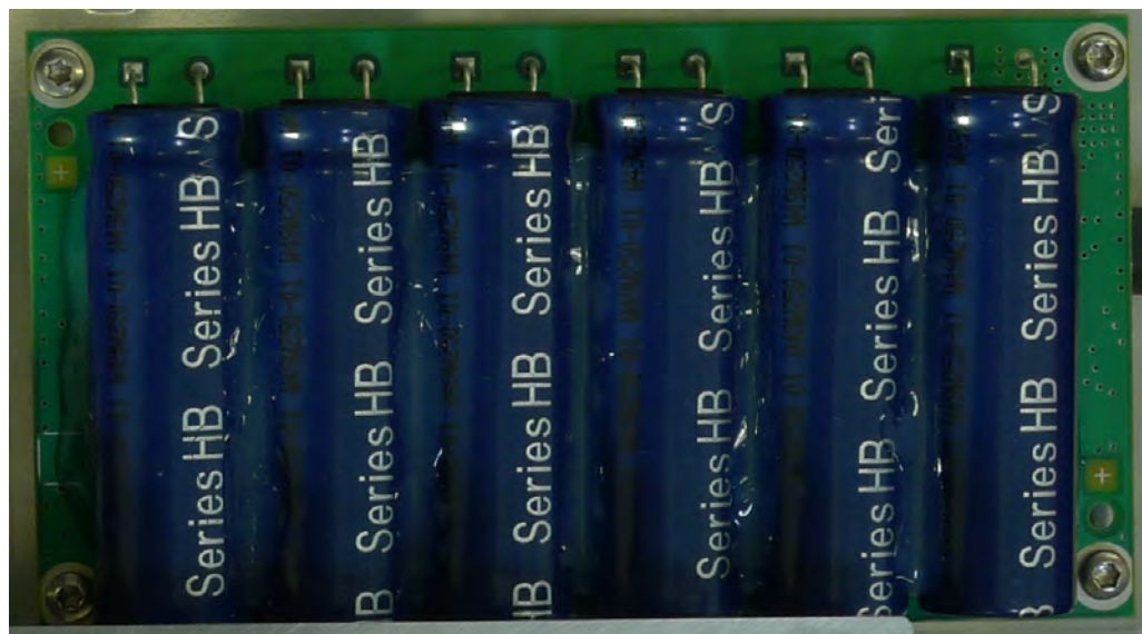
Figure 3-18: Capacitor Backup Battery
