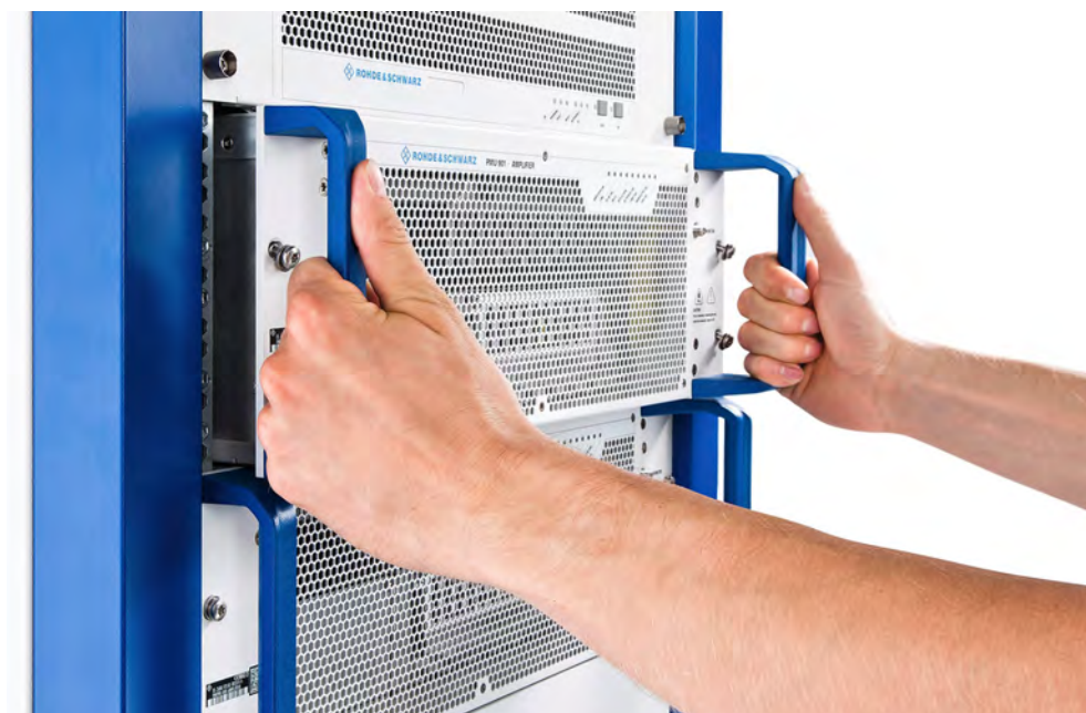
Fig. 3-11: Slide the amplifier into the rack
