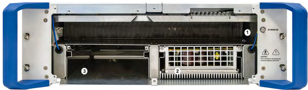
Fig. 5-2: Power supply unit and heat sink (front cover removed)
