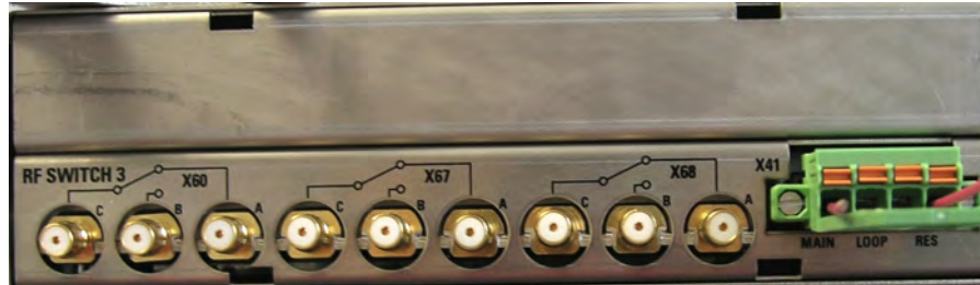
Fig. 3-17: RF loop plug X41 (LOOP) - RF Switch
