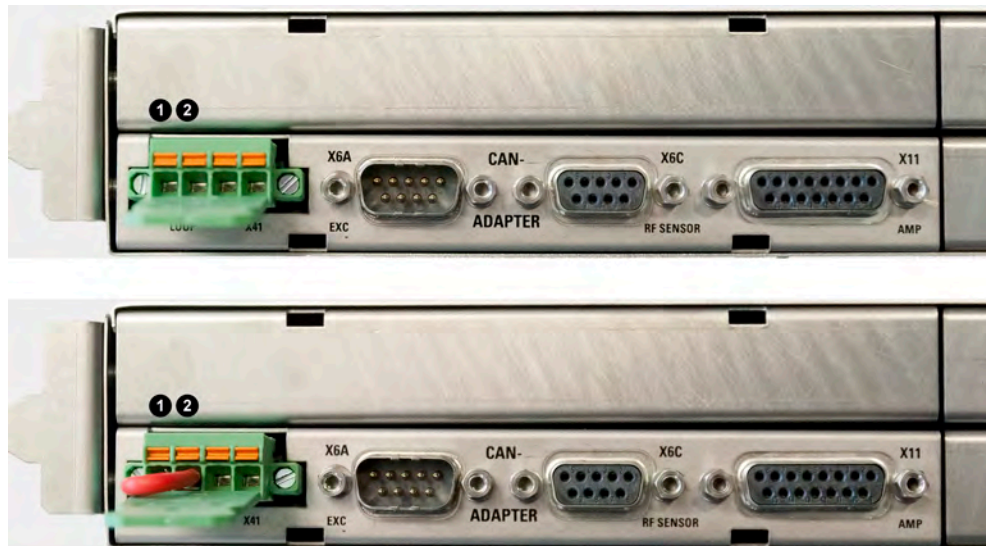
Fig. 3-16: RF loop plug X41 (LOOP), open and bypassed
