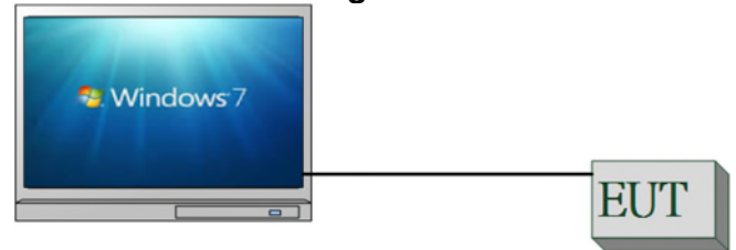
Fig. 2-2 Conducted (Antenna Port) Configuration
