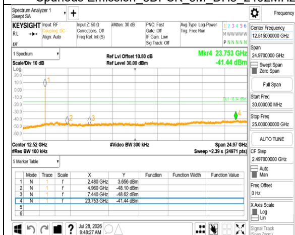
Spurious Emission 8DPSK 3M DH5 2480MHz
