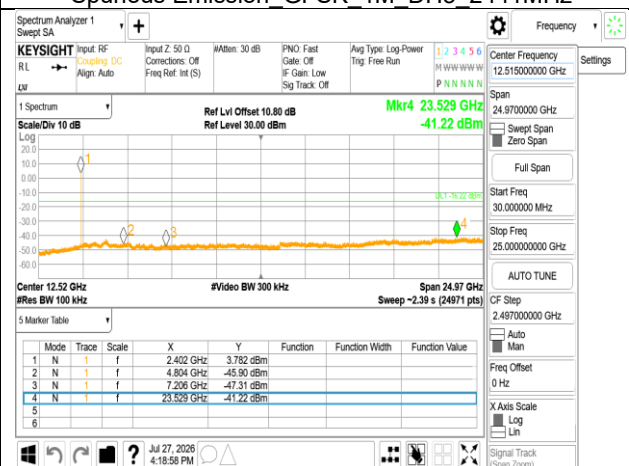
Spurious Emission 4DQPSK 2M DH5 2402MHz
