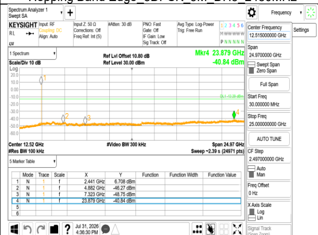
Spurious Emission GFSK 1M DH5 2441MHz
