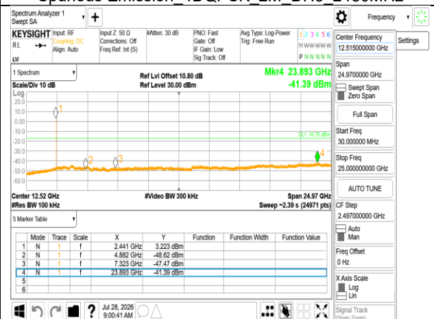
Spurious Emission 8DPSK 3M DH5 2441MHz
