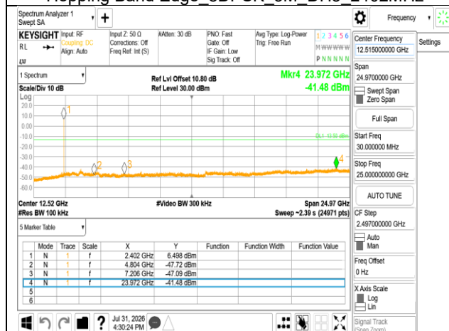
Spurious Emission GFSK 1M DH5 2402MHz
