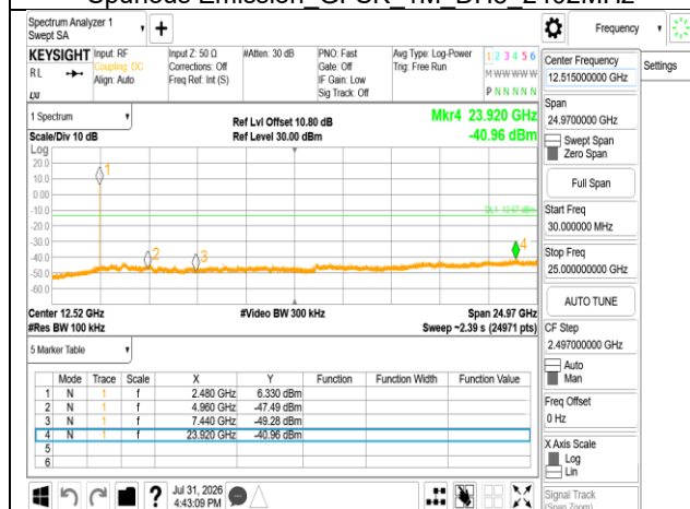
Spurious Emission GFSK 1M DH5 2480MHz
