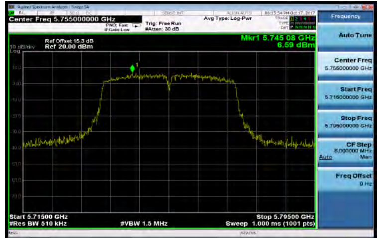
Peak Power Spectral Density Data Plot (CH High 5795 MHz)
