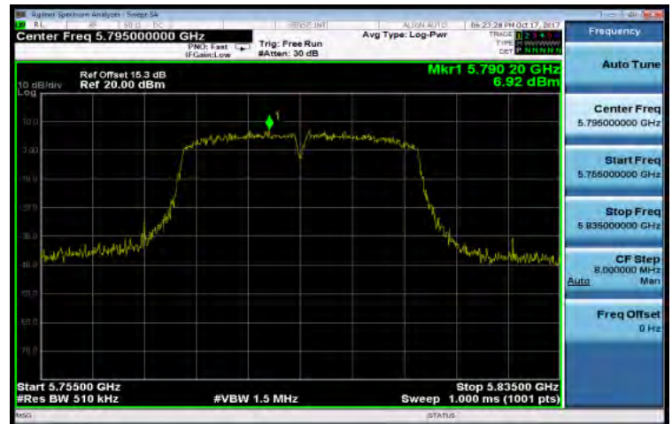
Peak Power Spectral Density Data Plot (CH High 5795 MHz)
