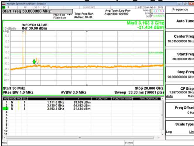
Spurious Emission\Band4 15MHz\QPSK RB1_0_CH20025
