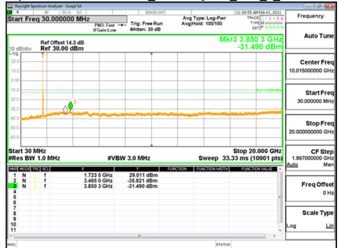
Spurious Emission\Band4 20MHz\QPSK RB1_0_CH20175
