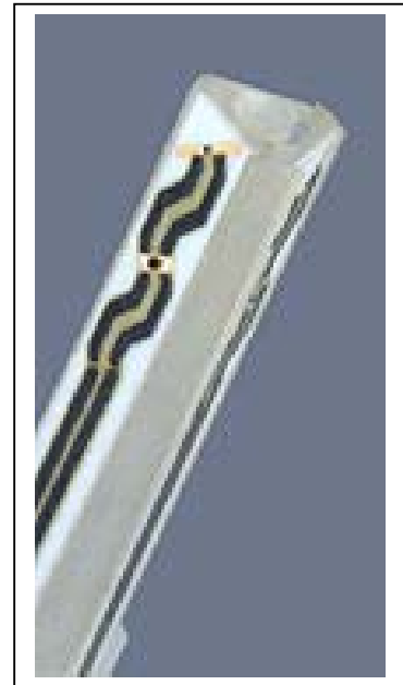
Inside view of ET3DV6 E-field Probe
