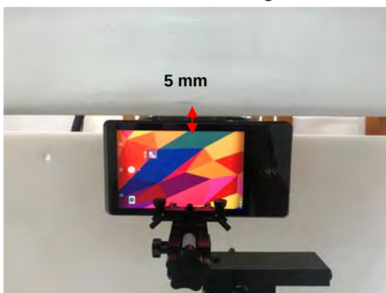
Fig.14 EUT Right side to flat phantom
