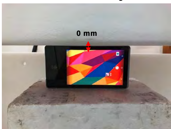
Fig.8 EUT Right side to flat phantom
