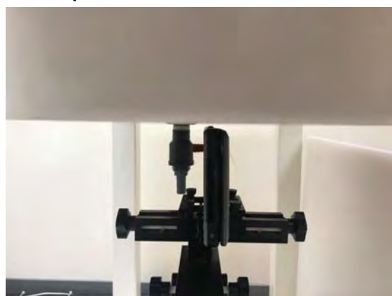
Fig.14 EUT Right side to flat phantom
