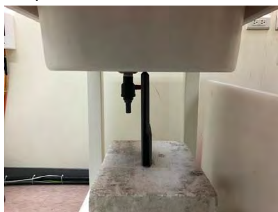
Fig.7 EUT Bottom side to flat phantom
