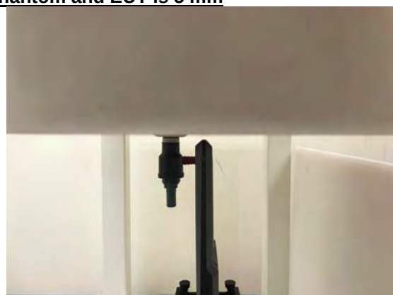
Fig.13 EUT Bottom side to flat phantom
