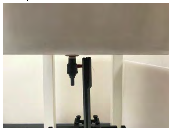
Fig.12 EUT Top side to flat phantom
