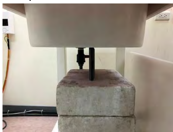
Fig.8 EUT Right side to flat phantom
