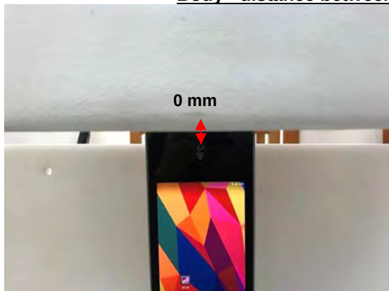
Fig.6 EUT Top side to flat phantom
