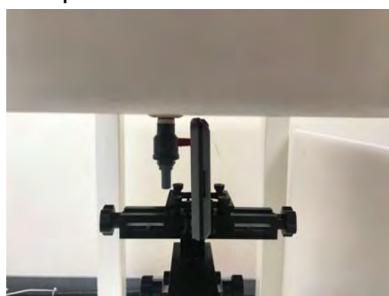
Fig.15 EUT Left side to flat phantom
