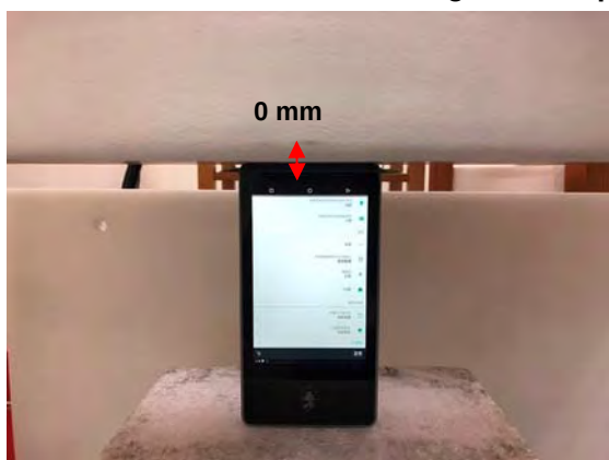
Fig.7 EUT Bottom side to flat phantom
