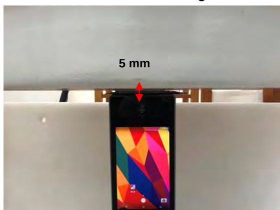
Fig.12 EUT Top side to flat phantom
