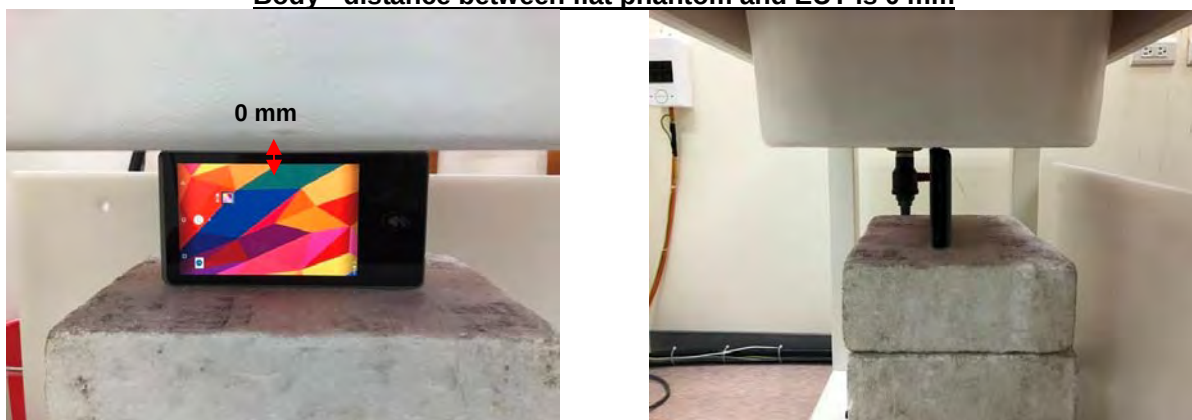
Fig.9 EUT Left side to flat phantom
