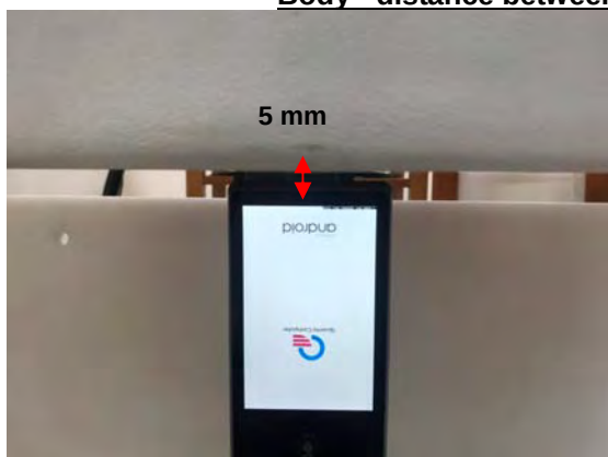
Fig.13 EUT Bottom side to flat phantom
