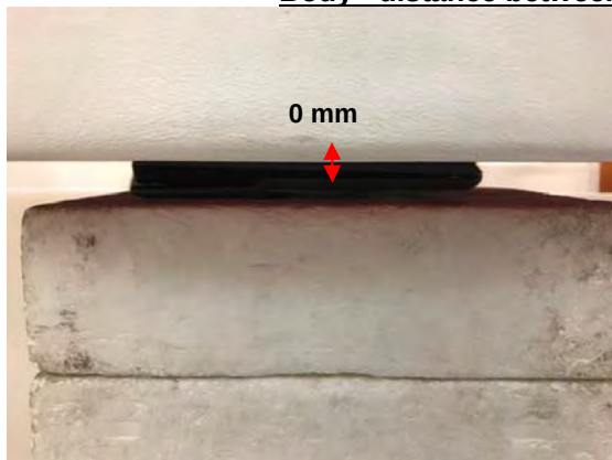
Fig.3 EUT Front side to flat phantom
