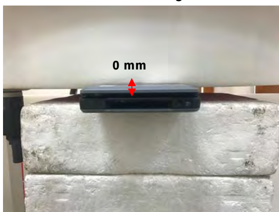
Fig.5 EUT Back side (WWAN) to flat phantom
