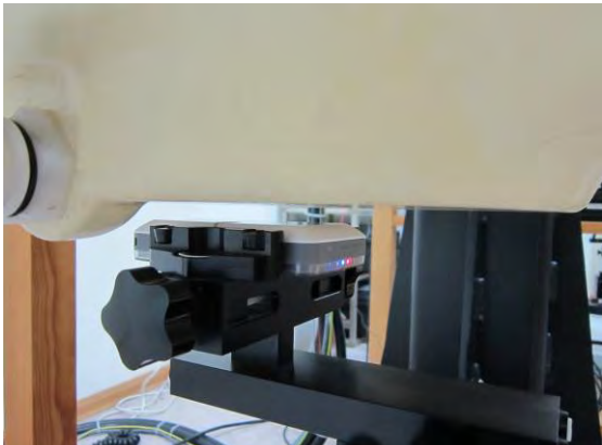
Fig.7 EUT Back to flat phantom
