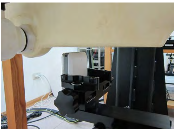
Fig.5 EUT Left to flat phantom
