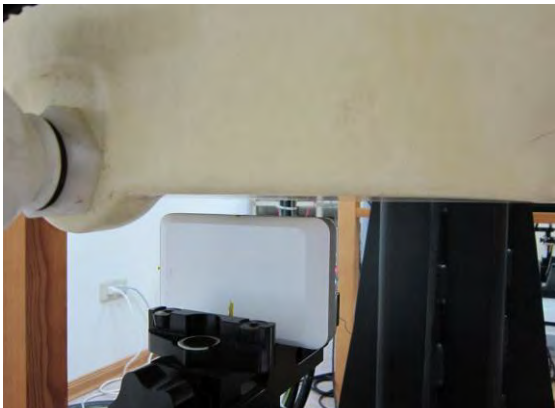
Fig.4 EUT Bottom to flat phantom
