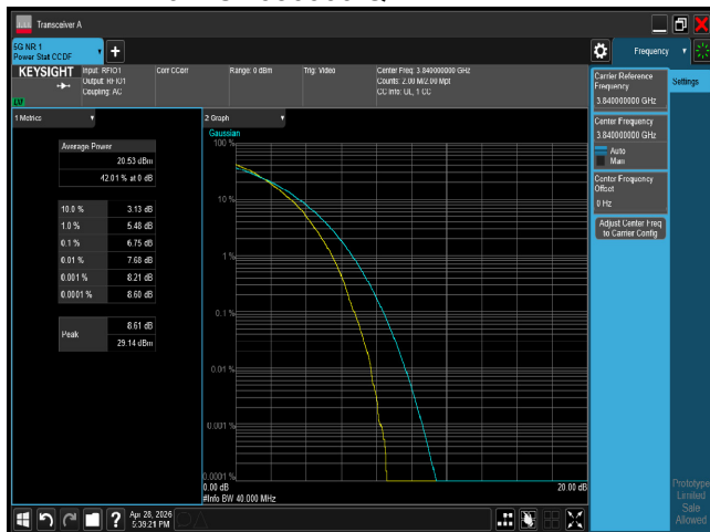
PTAR n77 40M CH656000 64QAM
