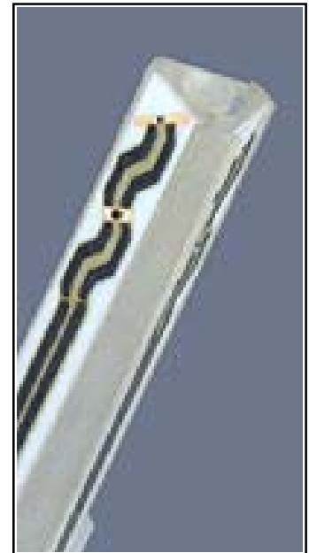
Inside View of ET3DV6 E-field Probe
