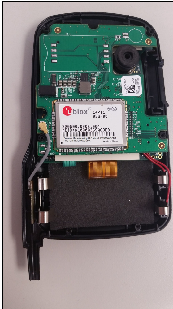
Figure 1: EUT Installed in Host
