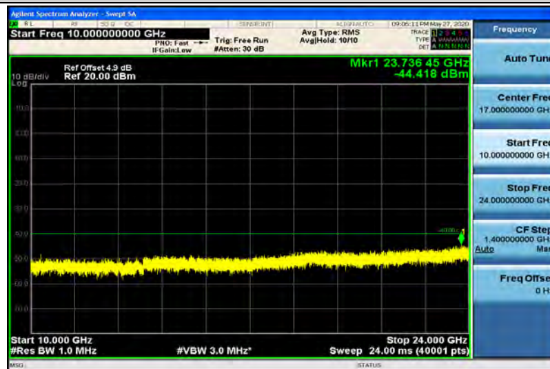
(Channel Bandwidth: 5 MHz)_HCH_QPSK_1RB#0-1
