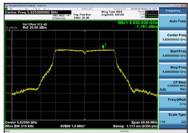
U-NII-3 Power spectral density-802.11 a(20MHz),5825MHz
