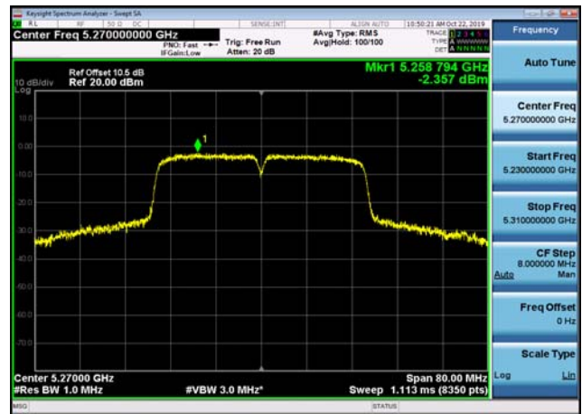
U-NII-2a Power spectral density-802.1 1ac(80MHz),5290MHz
