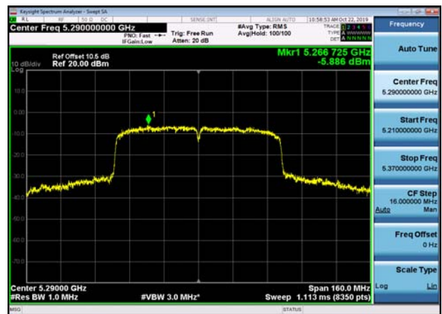
U-NII-2a Power spectral density-802.1 1ac(80MHz),5290MHz
