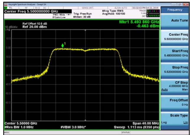
U-NII-2c Power spectral density-802.1 1a(20MHz),5700MHz
