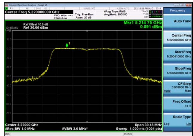
U-NII-1 Power spectral density-802.11 ac(40MHz),5190MHz
