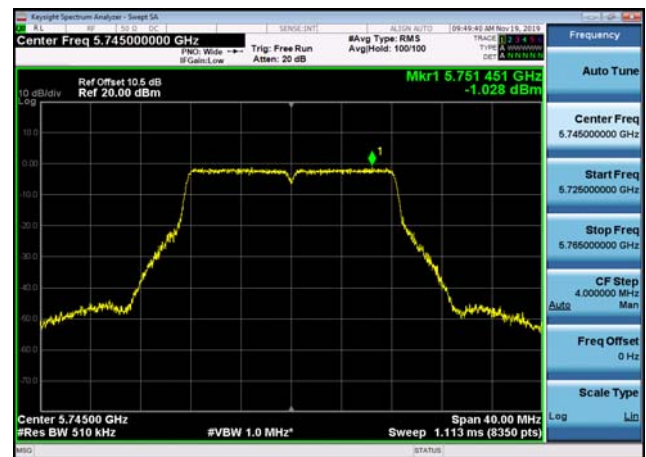
U-NII-3 Power spectral density-802.11 a(20MHz),5825MHz
