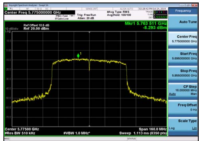
U-NII-3 Power spectral density-802.11 ac(80MHz),5775MHz
