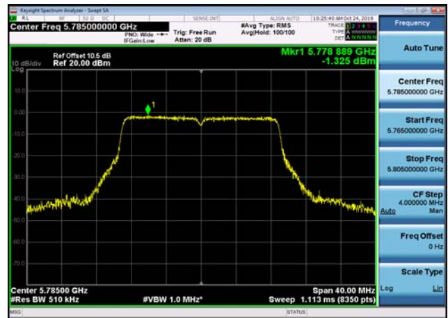
U-NII-3 Power spectral density-802.11 ac(40MHz),5755MHz
