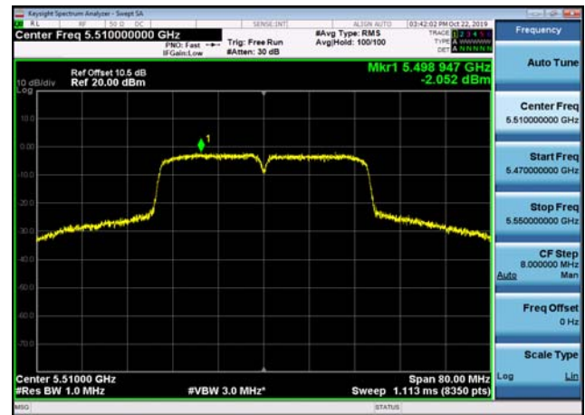
U-NII-2c Power spectral density-802.1 1n(40MHz),5670MHz
