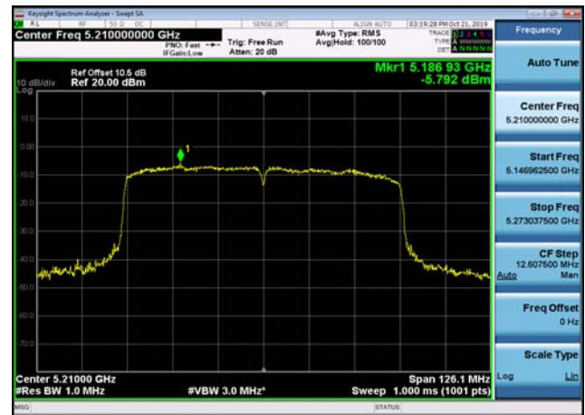
U-NII-2a Power spectral density-802.1 1n(20MHz),5300MHz
