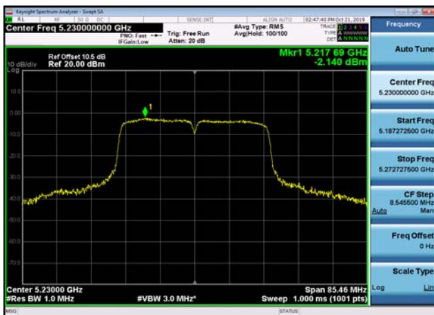
U-NII-1 Power spectral density-802.11 n(40MHz),5230MHz
