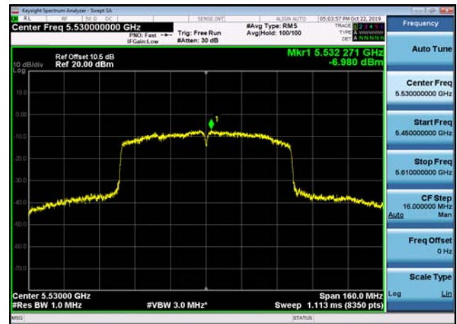
U-NII-2c Power spectral density-802.1 1ac(80MHz),5530MHz
