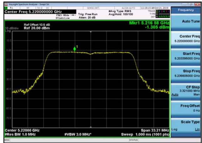
U-NII-1 Power spectral density-802.11 n(40MHz),5190MHz
