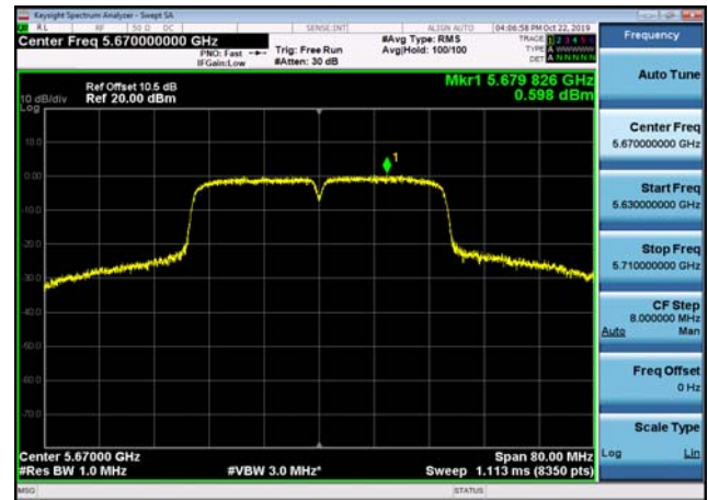
U-NII-2c Power spectral density-802.1 1a(20MHz),5600MHz
