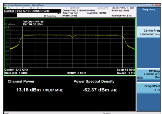
U-NII-1 Output Power-802.11a(20MHz) ,5180MHz
