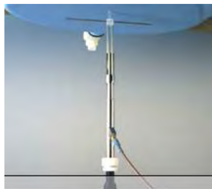
Photograph of the dipole Antenna
