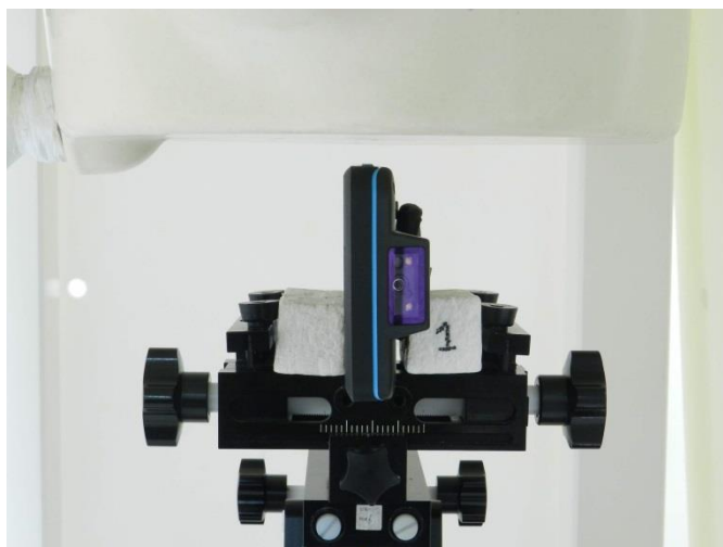
Left Side with Hand strap, Test Separation 10 mm
