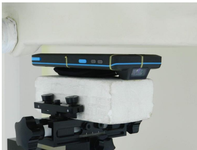
Front with Hand strap, Test Separation 10 mm
