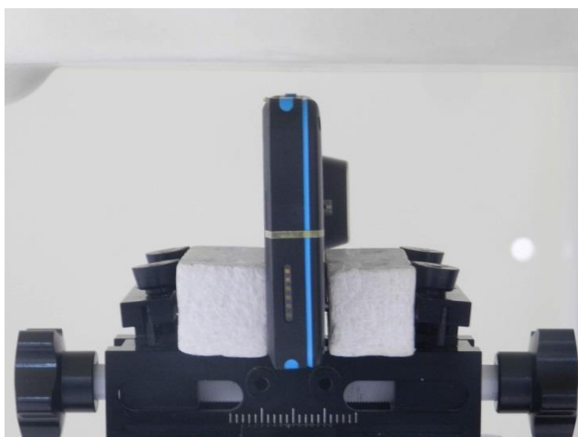
Right Side, Test Separation 10 mm
