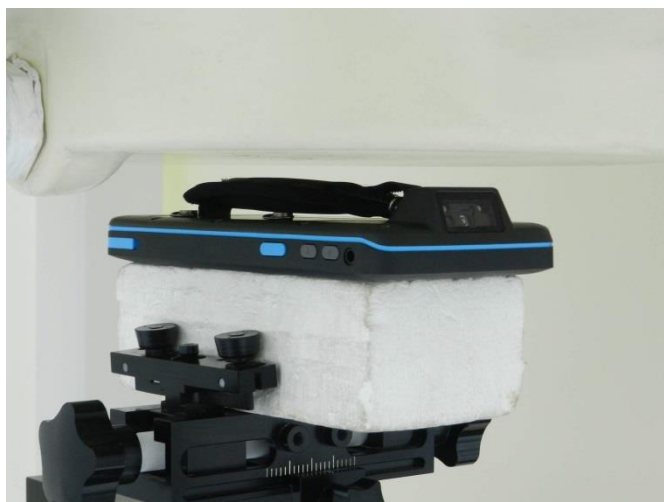
Back with Hand strap, Test Separation 10 mm
