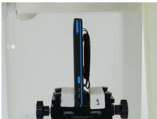
Bottom Side with Hand strap, Test Separation 10 mm
