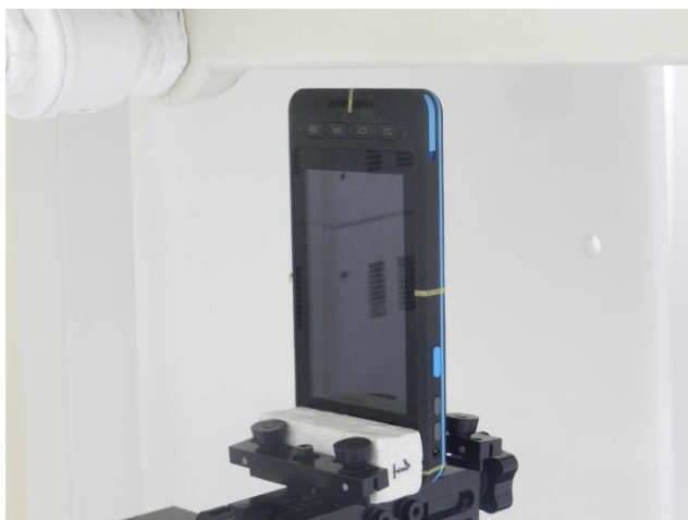
Bottom Side, Test Separation 10 mm
