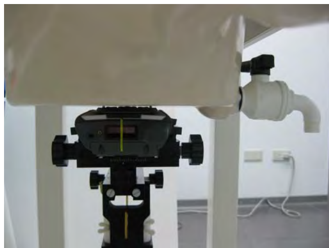
Fig.3.1 Front side of EUT is paralleled with flat phantom, separating 0cm between the back of the EUT and the flat phantom.
