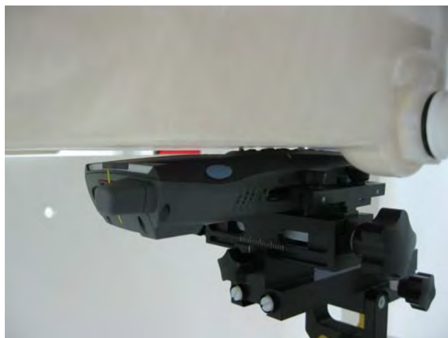
Fig.3.1 Front side of EUT is paralleled with flat phantom, separating 0cm between the back of the EUT and the flat phantom.
