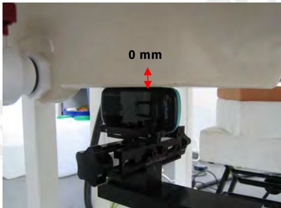
Fig.11 EUT Left side to flat phantom
