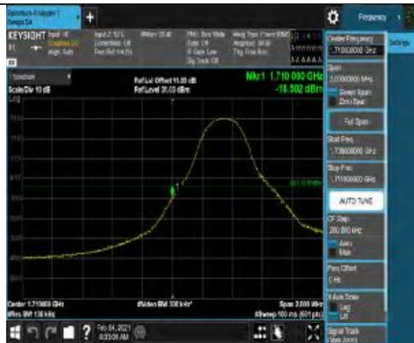
Band4-5MHz-64QAM-19975-1RB#24
