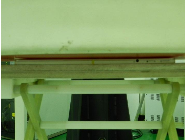
Bottom Face with Phantom 0 cm Gap
