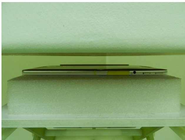
Back of Display Screen NB Mode with 2.5 cm Gap
