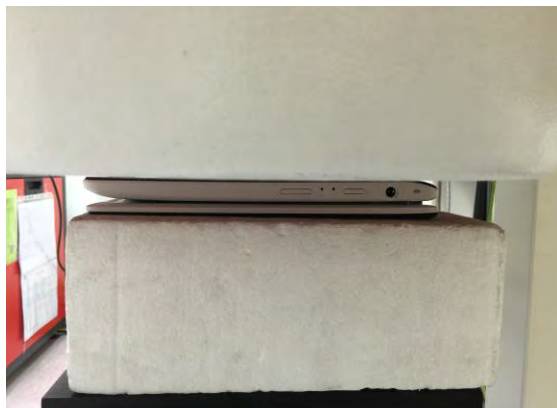
Fig.3 EUT Lap-held mode to flat phantom
