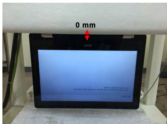
Fig.5 EUT Bottom side to flat phantom
