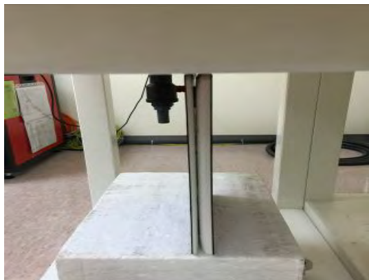
Fig.6 EUT Left side to flat phantom
