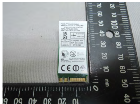
Fig 10 Integrate module (Model: QCNFA344A)
