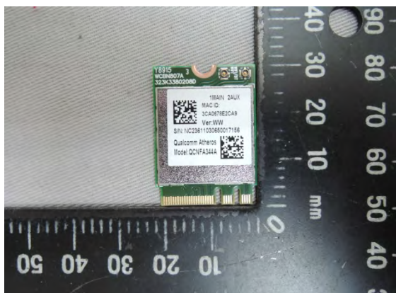
Fig 10 Integrate module (Model: QCNFA344A)
