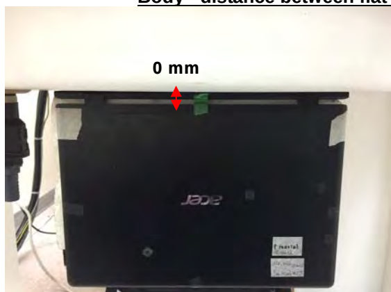
Fig.3 EUT Bottom side to flat phantom
