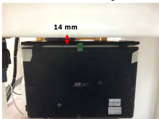
Fig.4 EUT Bottom side to flat phantom
