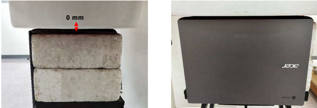
Fig.3 EUT Bottom side to flat phantom
