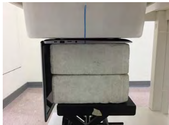
Fig.3 EUT Bottom side to flat phantom
