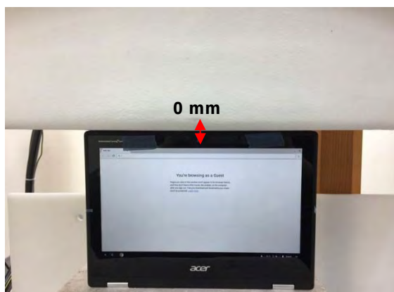
Fig.4 EUT Top side to flat phantom
