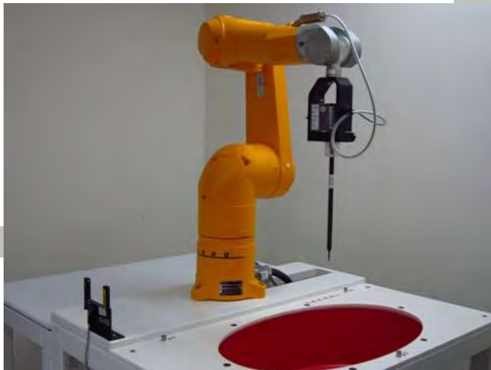
Fig.1 Photograph of the SAR measurement system
