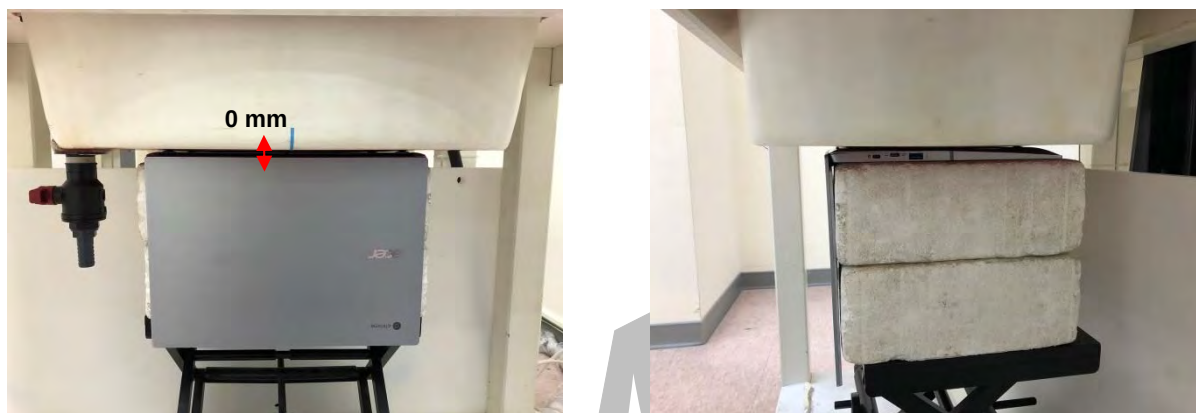
Fig.3 EUT Bottom side to flat phantom
