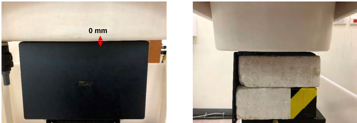
Fig.3 EUT Bottom side to flat phantom
