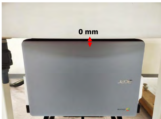
Fig.3 EUT Bottom side to flat phantom
