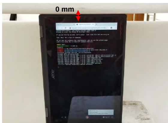
Fig.7 EUT Left side to flat phantom
