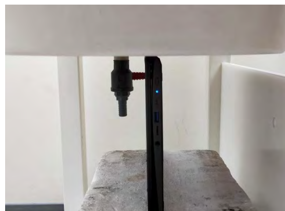
Fig.5 EUT Bottom side to flat phantom
