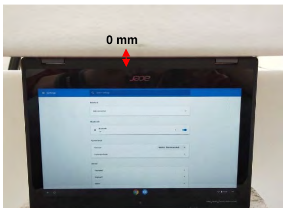
Fig.5 EUT Bottom side to flat phantom
