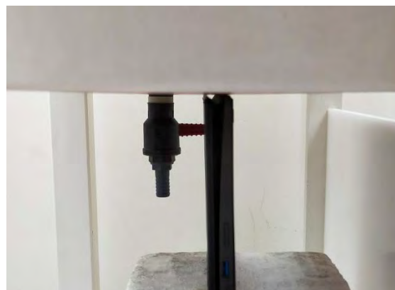
Fig.4 EUT Top side to flat phantom
