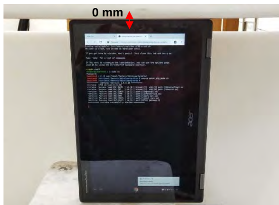
Fig.6 EUT Right side to flat phantom
