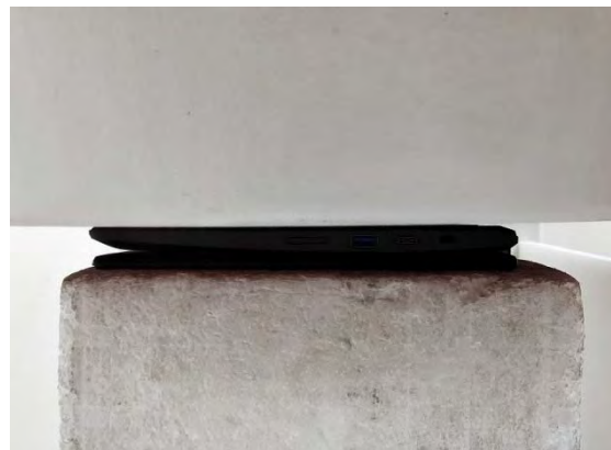
Fig.3 EUT Back side to flat phantom
