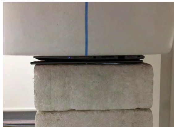
Fig.4 EUT Back side to flat phantom
