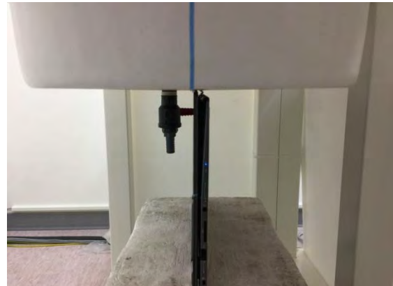
Fig.3 EUT Top side to flat phantom
