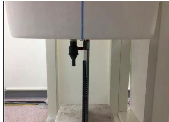
Fig.6 EUT Right side to flat phantom
