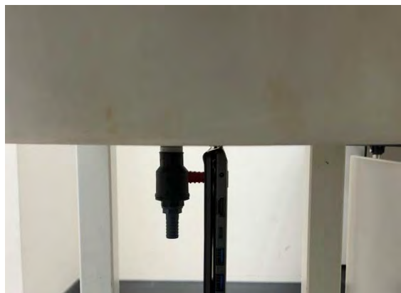
Fig.5 EUT Bottom side to flat phantom
