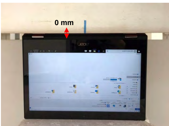
Fig.5 EUT Bottom side to flat phantom
