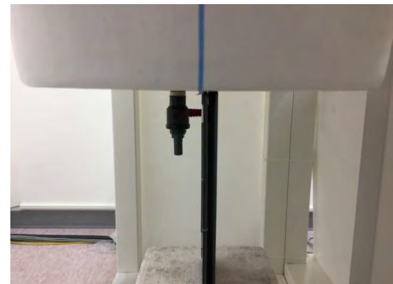
Fig.7 EUT Left side to flat phantom
