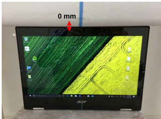
Fig.3 EUT Top side to flat phantom
