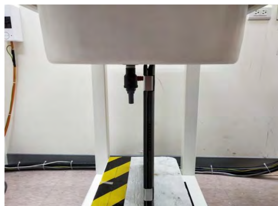
Fig.6 EUT Right side to flat phantom
