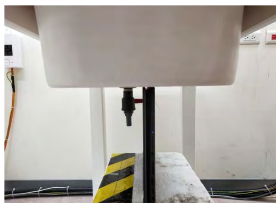
Fig.4 EUT Top side to flat phantom
