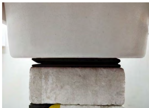
Fig.3 EUT Back side to flat phantom
