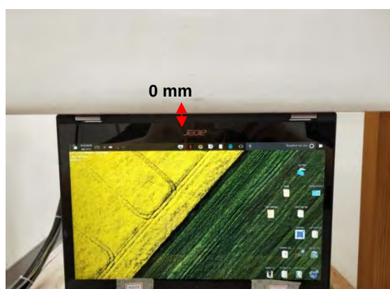
Fig.5 EUT Bottom side to flat phantom
