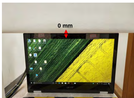
Fig.4 EUT Top side to flat phantom
