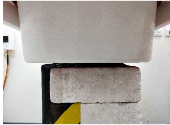
Fig.3 EUT Bottom side to flat phantom
