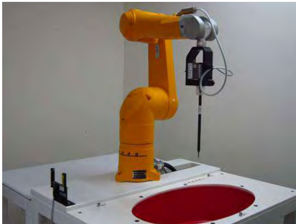
Fig.1 Photograph of the SAR measurement system
