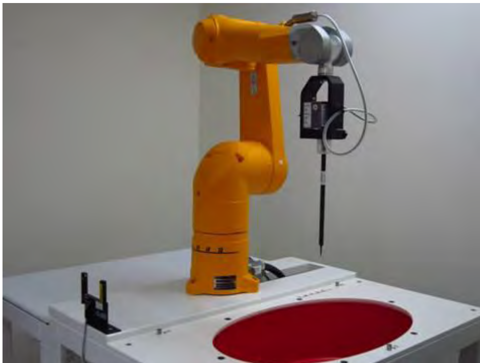
Fig.1 Photograph of the SAR measurement system
