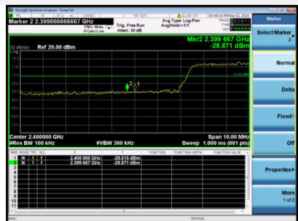
802.11ax-20 MHz(SU) LOW CHANNEL, BAND EDGE
