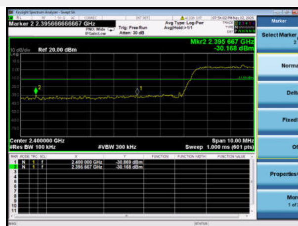
802.11ax-20 MHz(SU) LOW CHANNEL, BAND EDGE
