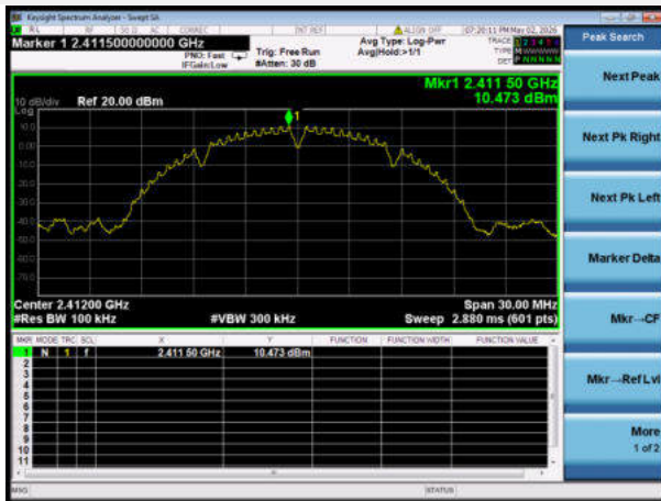
802.11b LOW CHANNEL, CARRIER LEVEL
