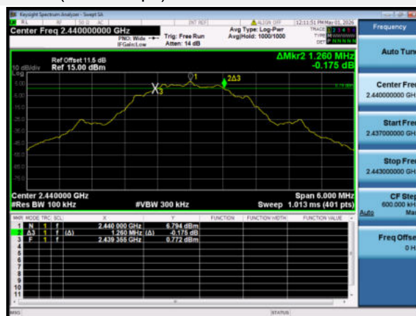
GFSK (BLE 2Mbps) MIDDLE CHANNEL
