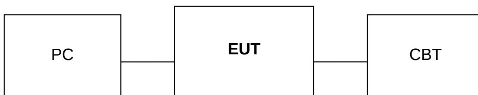
Fig. 2-2 Conducted (Antenna Port) Configuration
